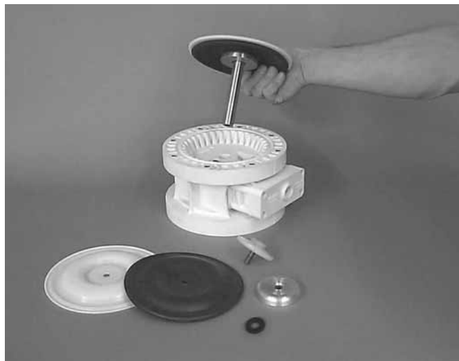
Step 10. Figure 10 After loosening and removing the outer piston the diaphragm assembly can be disassembled.
